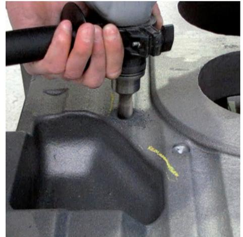
Preparing for weld by drilling
