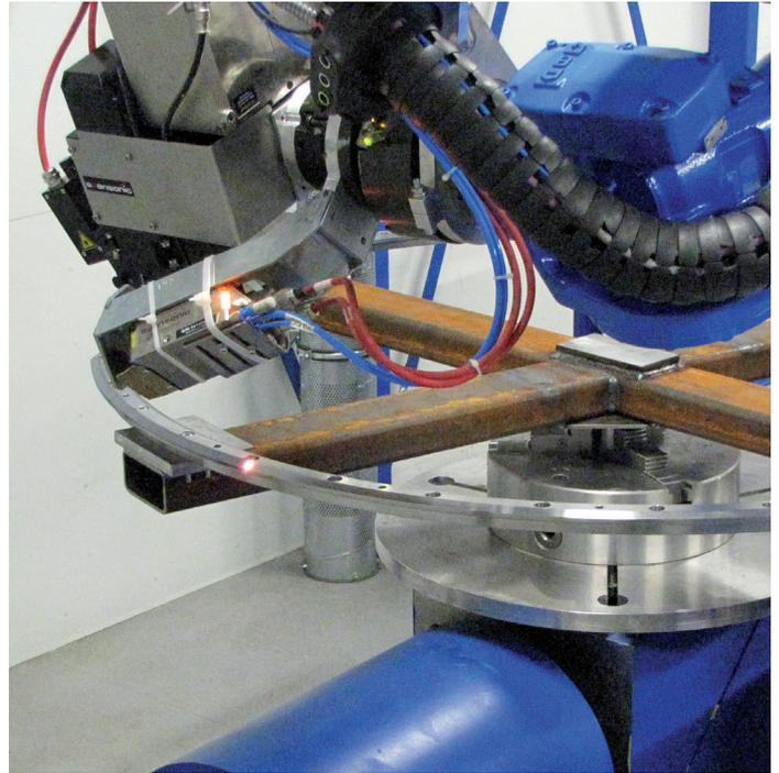
We are able to harden rotary parts of large diameters.
