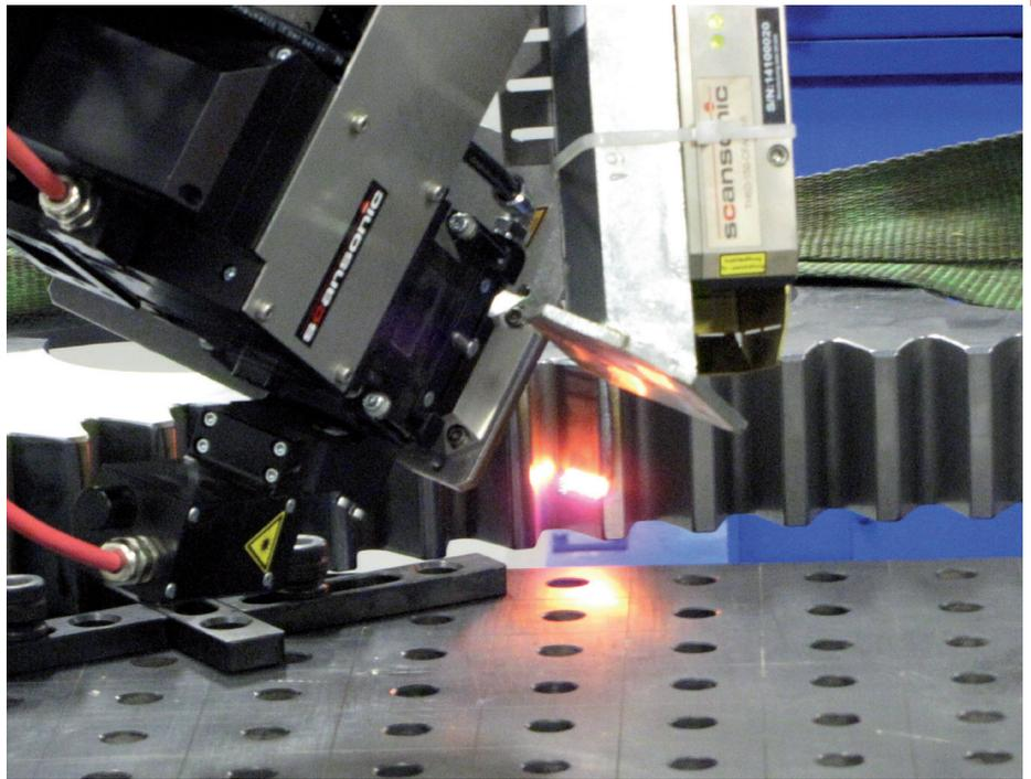
We can harden sides of tothing from a module of 4 mm.
