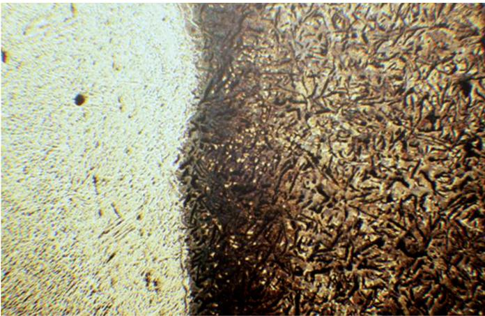
Arc welding using E-5716 electrode (50%Ni), 4 layers, calking and brushing of each layer; waiting for the cooling of each layer – about 40 min.
