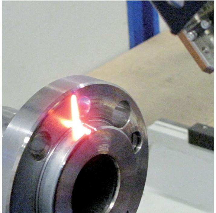
Due to this scanning technology the temperature is controlled locally, which ensures optimal hardening temperature and prevents partial melting of edges.
