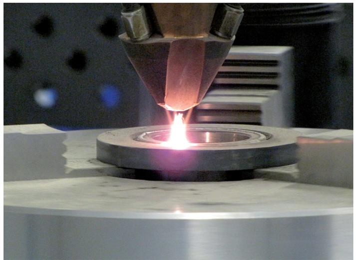
The six-axis robotic arm allows us to process components of complex shapes. The technology of alloy cladding is used to repair worn parts of moulds and various other parts.
